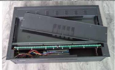
6. Plug the power cord into an electrical outlet to test the unit before reinstalling in or on wall.
