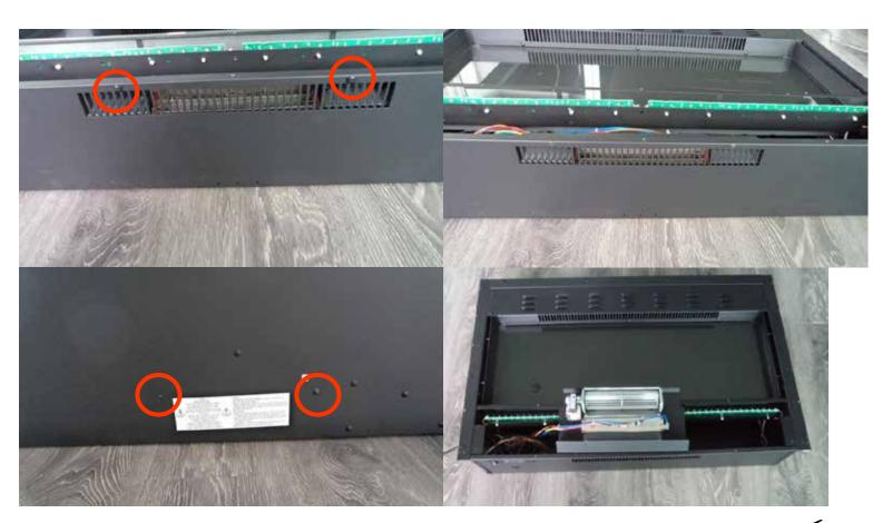
4. Unplug all the wires from the PCB board.
